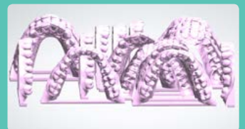
3D Printer Integration with automatic nesting
